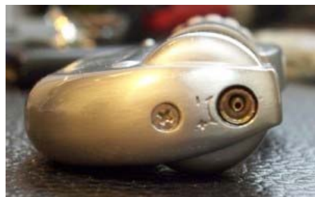
Fill port and flame adjuster
